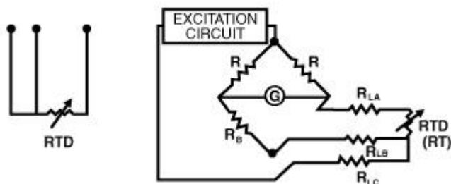
Industrial sensors commonly use this three wire connection system. For this system to be effective, all the leads ( $R_{LA}$ , B, C) should be very near the same length and of the same gauge.
