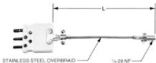
Figure 3 Nozzle Bolt with Stainless Steel Overbraided Extension
