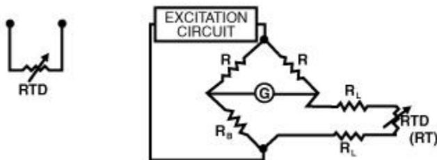
At balance  $R_B$  will equal  $R_T + 2R_L$  giving an error equal to the two leads of the sensor connection. Depending on lead length and wire size the error may be negligible or profound.
