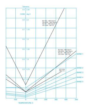
Table 3 illustrates the tolerances applicable for specifications DIN 43760 - 1980, BS 1904 : 1984, IEC 751 : 1983 and JIS C1604 - 1981, together with the Thermo Sensors Bands 1 to 5.
