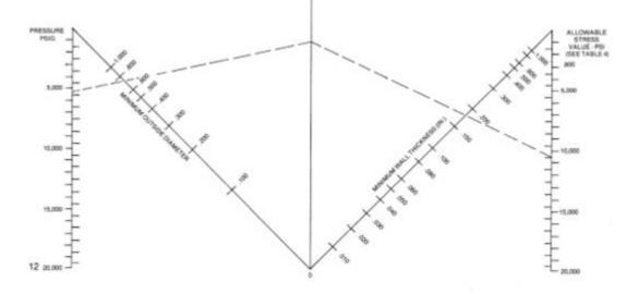
The Nomograph and Table 4 below may be applied in calculating wall thickness. The following example demonstrates the use of the nomograph in a typical problem situation.
