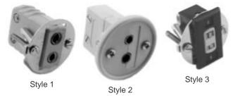
Single circuit jacks designed for mounting into control panel or instrument case can be wired and installed completely from the front. Fits in standard 3/4" knockout (1 1/8" diameter). Permanently attached self-fastening device simplifies mounting, holds tight.
