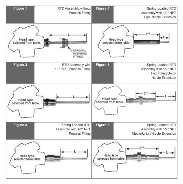
\* For custom extension length, add desired length as suffix to basic order code. Variable lengths only available in figure 4, 5 and 6 Example: 5046, for 6" long extension.
