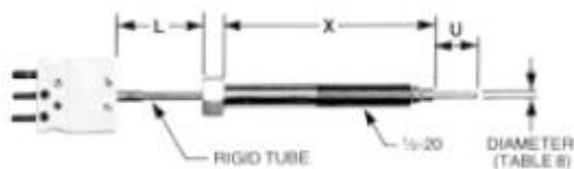
Figure 2 Immersion Bolt with Rigid Tube Extension
